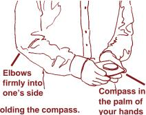
Fig. 2. Holding the compass.
